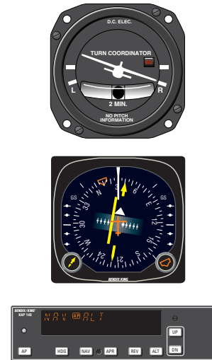
3. When the computed capture point is reached, the HDG annunciation changes to NAV and a right turn is initiated by the autopilot.
