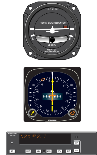
4. The turn is complete and the autopilot is tracking the GPS course.
