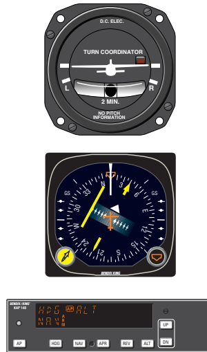
2. GPS data is selected for the HSI. The course pointer is set to 040°. The NAV button is depressed and NAV ARM is annunciated.
