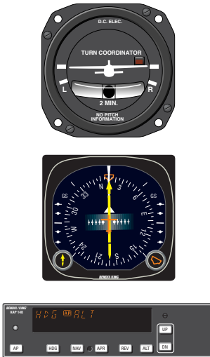
1. Continuing on heading 010°, a GPS waypoint is established. A 30° intercept is desired.
