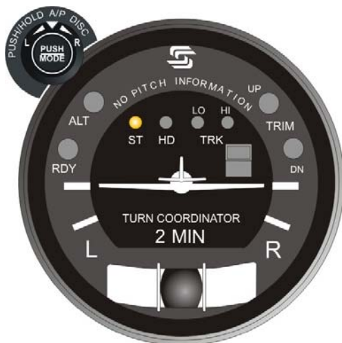
Fig. 2-21. AP Display, ST Mode Engaged (System Thirty)
