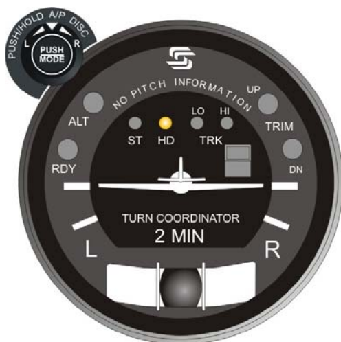
Fig. 2-22. AP Display, HD Mode Engaged (System Thirty)
