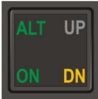
Fig. 2-30. ALT HOLD ON/OFF Switch Display, ALT HOLD Mode Engaged, TRIM DN Required (System Thirty ALT)
