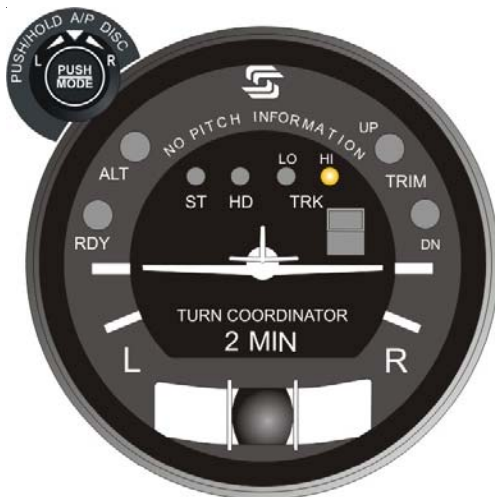
Fig. 2-20. AP Display, HI TRK Mode Engaged (System Twenty)
