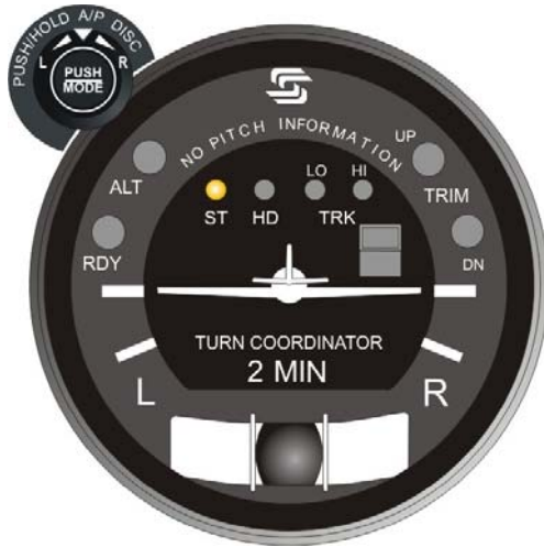
Fig. 2-17. AP Display, ST Mode Engaged (System Twenty)
