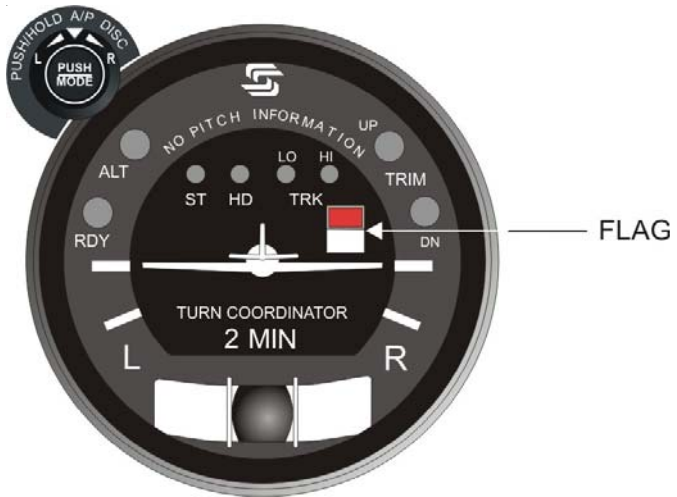
Fig. 2-12. AP Display, Low Voltage Flag (System Thirty)
