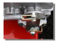
Attach the other end of the spring clip onto transmission brake lever. Use the 1/4" bolt from brake lever and secure with nut – leave room for clip to move freely.
