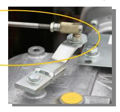
Attach end of shift cable by pulling back outer sleeve and slip on to the transmission shifter
