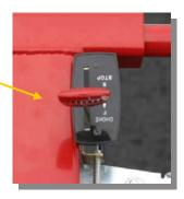
Locate the throttle control attached to the engine and bring it up to top of handle. Remove the two Phillips Screws on side of handle and install throttle control.
