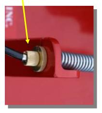
**Step 3 – Brake Cable** Locate cable from brake handle at top of machine. Follow down to spring end. Line up the slots in brass fitting in order to slip wire into bracket. Pull back the spring over the cable and slip wire into lined up slots on support. Turn slots to keep in place
