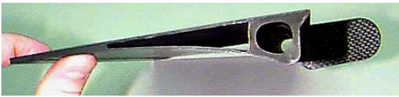
Figure 8 – Resin-transfer-molded (RTM) flap
